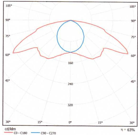
Due to missing symmetry properties, no UGR table can be displayed for this luminaire.
